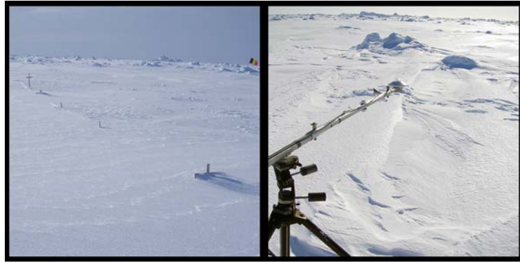
Fig. 10 : (left) The Brussels “Cimetière d’Ixelles” albedo line. (right) Typical position of the pyranometer on the line.
