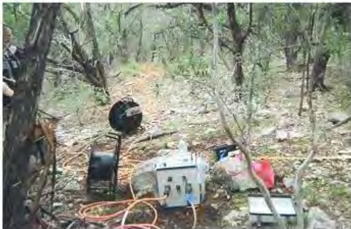
Figure 1a. The set up of the line once the conductive wires are set into place, in line with the electrodes. The meter and battery are located at the bottom center and right.
