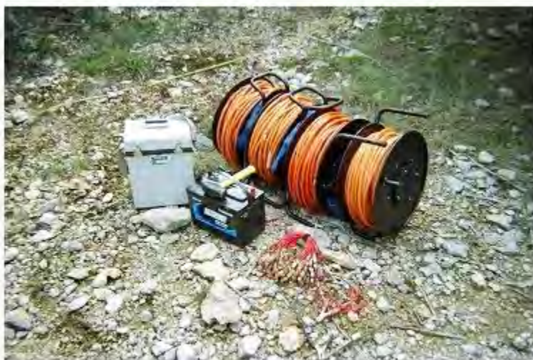
Figure 1b. Materials used: From top left to right are the meter, the conductive cables, the battery, the hammer and the connector cables.
