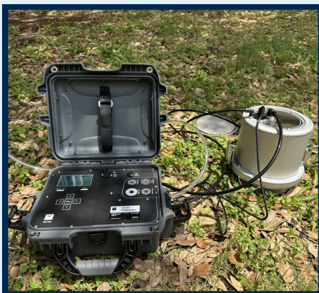
METER SATURO automated saturated hydraulic conductivity meter
