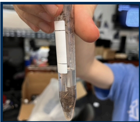
A soil dilution before suspension in a 15ml centrifuge tube
