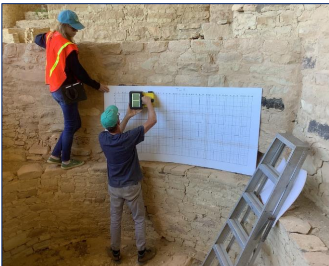
View of a radar survey in a ceremonial kiva, conducted by Blake Weissling, assisted by Sara Rodriguez.
