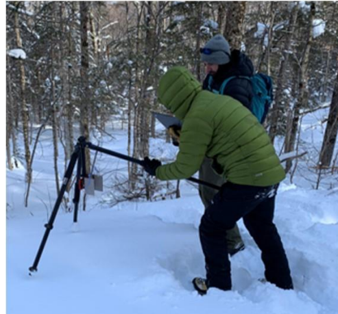
Radar measures snow depth
